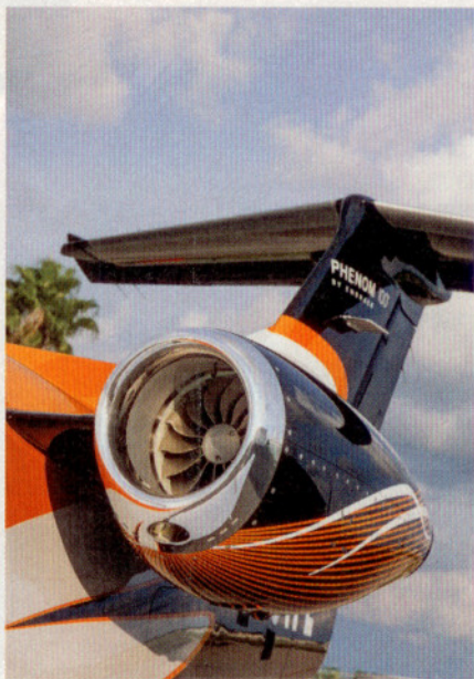
NEW FOR 2013 will be an optional side-facing seat across from the cabin entry door (above left), as seen in a photo taken at the new Melbourne assembly facility. The 1,695 lbst Pratt & Whitney PW617 engines (above right) can go to 1,820 lbst under its automatic power reserve (APR) mode in emergencies such as an engine failure after takeoff.
